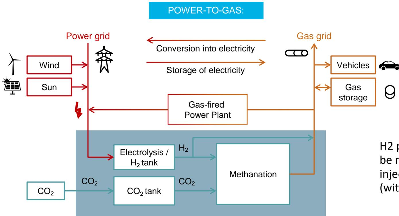
H<sub>2</sub> produced by P2G could be methanised or directly injected in the existing grid (with limits)
